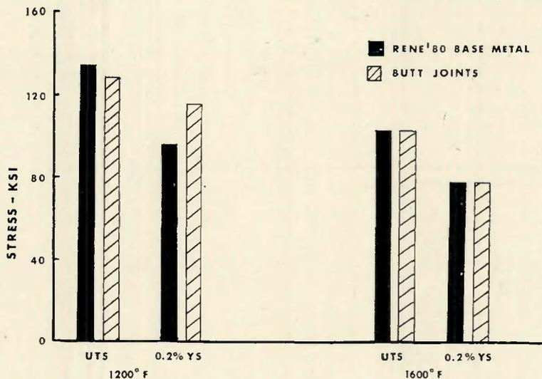
Fig. 3—Tensile properties of activated diffusion bonded butt joints in René 80 vs. those of the base metal
