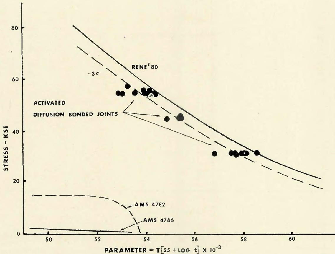
Fig. 4—Stress rupture properties of activated diffusion bonded joints in René 80 compared with those of conventional brazed joints
