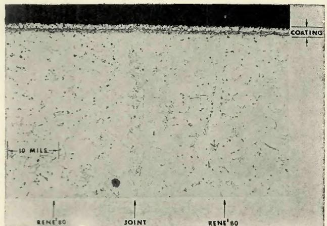
Fig. 6—Activated diffusion bonded joint in René 80 after coating and static oxidation at 1800° F
