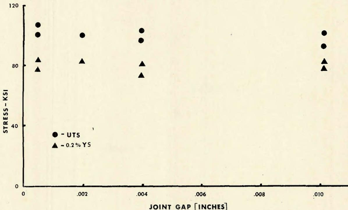
Fig. 7—Effect of joint gap on 1600° F tensile properties of activated diffusion bonded butt joints in René 80
