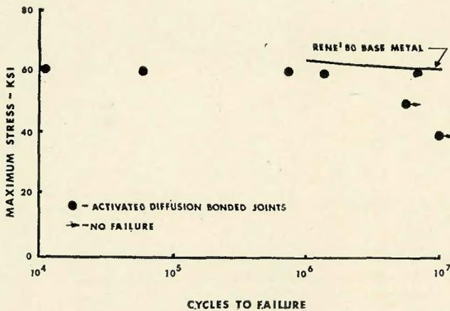
Fig. 5—1400° F high cycle fatigue strengths of activated diffusion bonded butt joints in René 80
