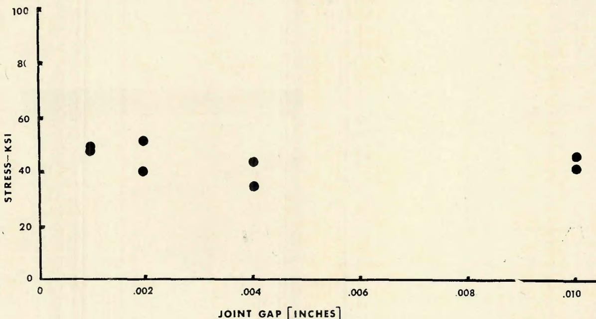
Fig. 8—Effect of joint gap on 1600° F/50 hr stress rupture properties of activated diffusion bonded butt joints
