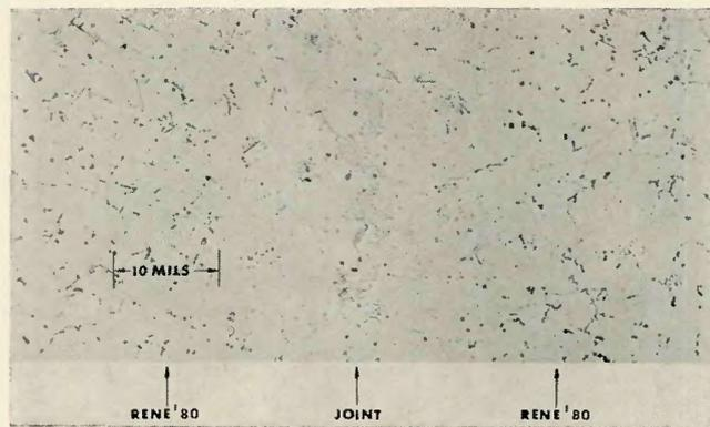
Fig. 2—Typical activated diffusion bonded joint in René 80
