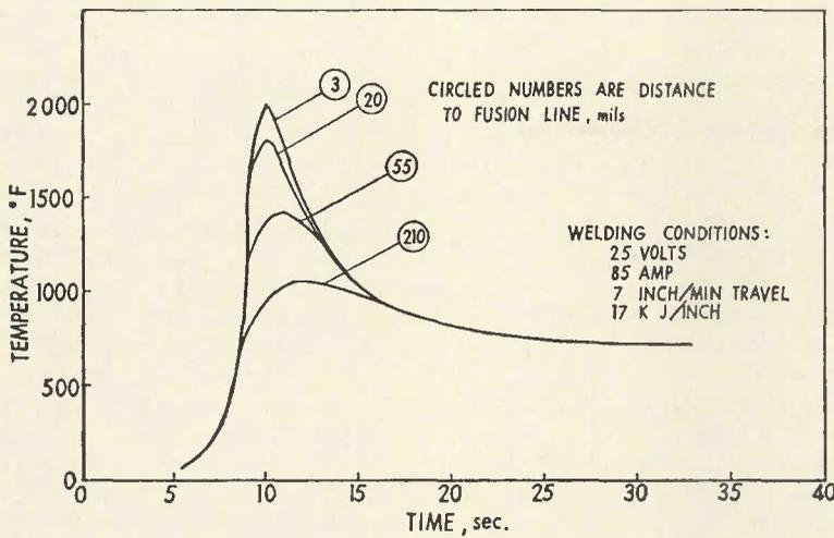
Fig. 1—Thermal cycles experienced by the heat-affected zone of 3/8 in. thick CA715 alloy plate
