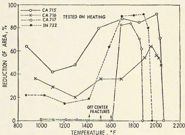
Fig. 2—Hot ductility data representing "On Heating" test conditions
