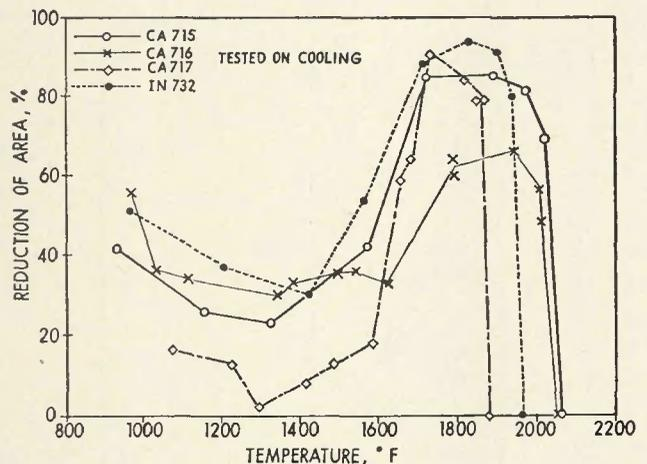
Fig. 3—Hot ductility data representing "On Cooling" test conditions
