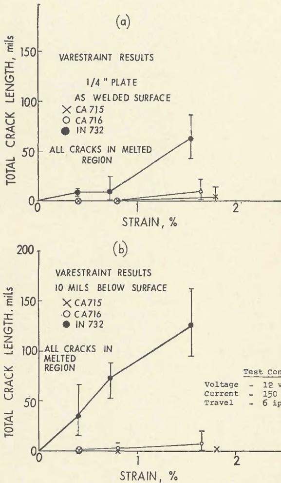
Fig. 5—Varestraint test results for modified copper-nickel alloys
