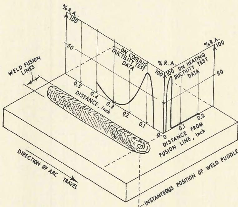
Fig. 4—Relationship between plots of "On Heating" and "On Cooling" hot ductility test data with respect to a bead-on-plate weld for CA717 alloy
