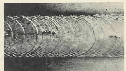
Fig. 6—The appearance of Varestraint weld beads supplementally protected with a trailing shield. A (left)—IN732 alloy; B (center)—CA716 alloy; C (right)—CA715 alloy. X4 (reduced 28% on reproduction)
