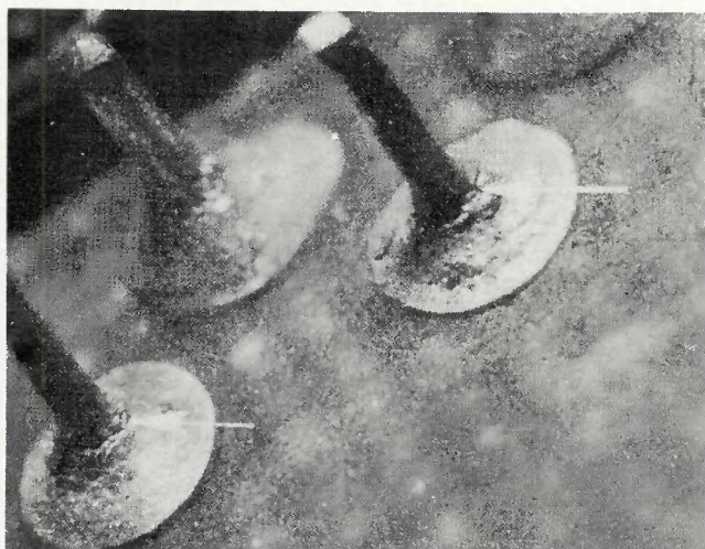
Fig. 6 — Low stress high cycle failure. (Left) note the rough solder surface caused by many small joint deflections. (Right) note recrystallization in the high stress areas of the solder joint
