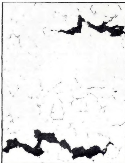
Fig. 8 — Sigma phase (dark-etching constituent) in Type E308 stainless steel deposit fractured after 600 h at 1200 F with less than 1% total elongation. Etchant: 10N KOH. Mag. X750, reduced approx. 41%
