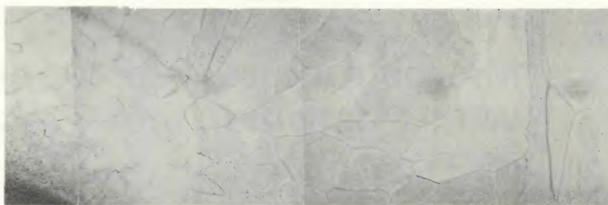
Fig. 2 — Overall view of the GTA welded Ti-6Al-6V-2Sn microstructure using matching filler metal (X35, reduced 54%)
