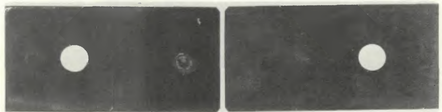
(a) Shear at weld.
