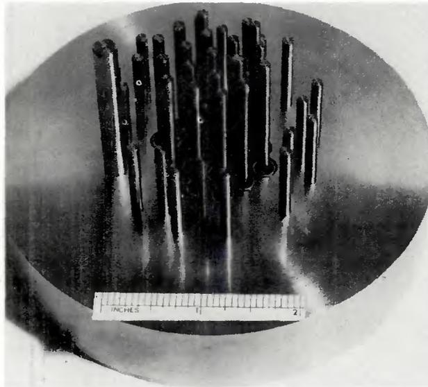
Laser welded reactor fuel element prototype
