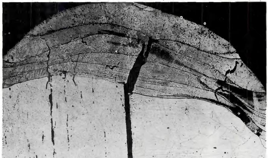
Fig. 14 — Severe cracking in a laser welded austenitic stainless steel tube-to-header joint (X100, increased 24%)
