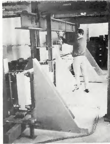
Fig. 5 — The lateral support and loading systems
