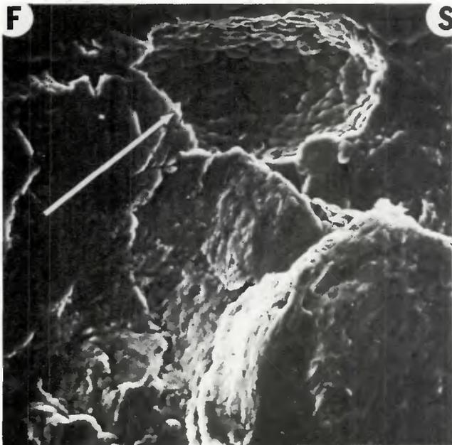
Fig. 9 — Plan view of another of the pores (arrow) responsible for the fatigue fracture surface shown in Fig. 7 (see Fig. 6 for location). FS is one edge of the fracture surface. (X580, reduced 9%)
