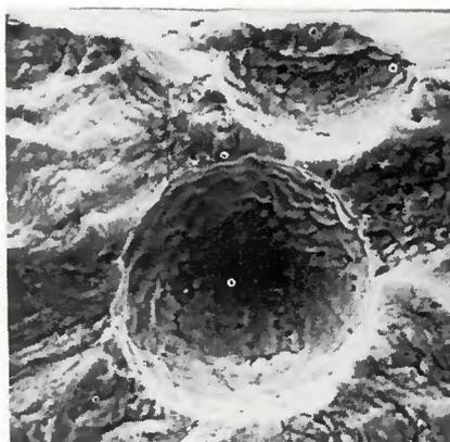
Fig. 5 — Higher magnification view of the two pores shown in Fig. 4. (X525, reduced 41%)
