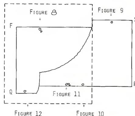
Fig. 6 — Diagrammatic representation of the fracture surface in Fig. 7 (broken line shows actual boundary). Magnified views of the pores are shown in the subsequent figures indicated
