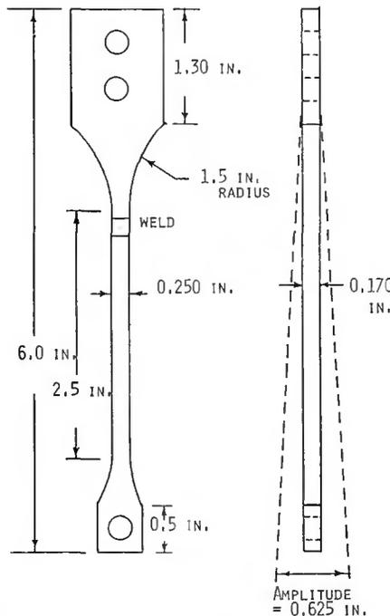
Fig. 2 — Shape and dimensions of the flexural bending fatigue testpiece, showing also the deflection amplitude employed
