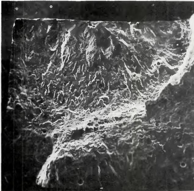
Fig. 7 — Plan view of a portion of the fracture surface of a fatigue testpiece from the fastest Series C weld. Note the large number of pores visible on the fracture surface. Welding speed = 50 ipm (2.11 cm/sec); angle of tilt = zero. (X 22, reduced 9%)
