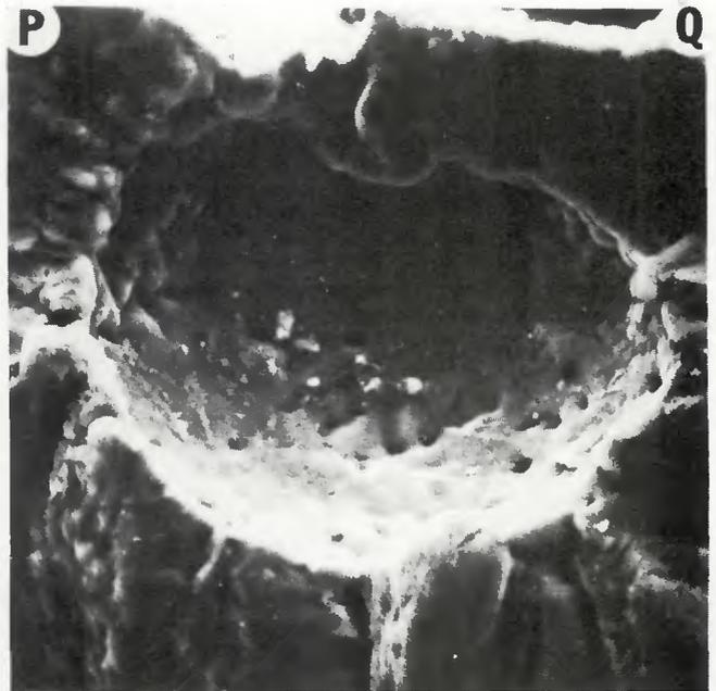
Fig. 12 — Plan view of another pore responsible for the fatigue fracture surface shown in Fig. 7 (see Fig. 6 for location). PQ is one edge of the fracture surface. (X1100, reduced 9%)
