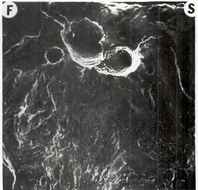
Fig. 8 — Higher magnification view of one of the group of pores responsible for the fatigue fracture surface shown in Fig. 7 (see Fig. 6 for location). FS is one edge of the fracture surface. (X220, reduced 9%)
