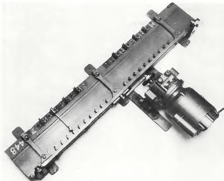
Fig. 3 — The flexural bending fatigue equipment showing one testpiece in place
