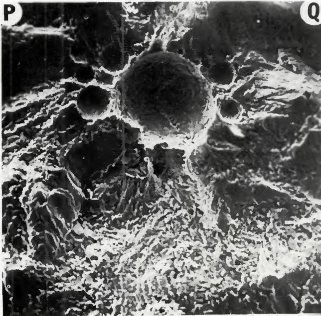
Fig. 11 — Plan view of a third group of pores responsible for the fatigue fracture surface shown in Fig. 7 (see Fig. 6 for location). PQ is one edge of the fracture surface. (X230, reduced 9%)
