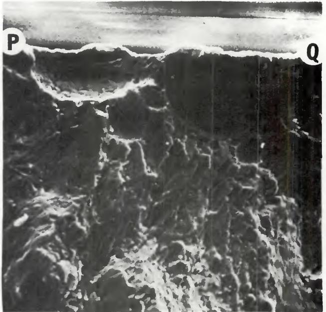
Fig. 10 — Plan view of a second group of pores responsible for the fatigue fracture surface shown in Fig. 7. (see Fig. 6 for location). PQ is one edge of the fracture surface. (X370, reduced 9%)
