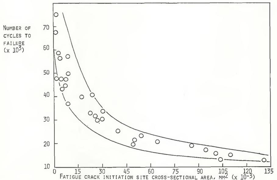
Fig. 13 — Number of cycles to failure of the flexural bending testpieces versus the related fatigue crack initiation site cross sectional area.
