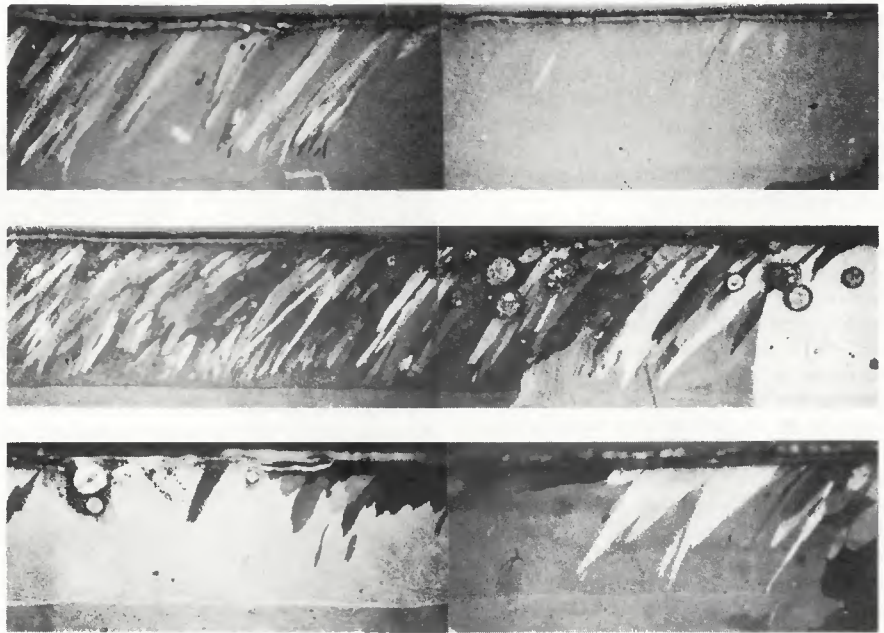
Fig. 7 — Fusion zone of a single specimen displaying a spectrum of growth structures, 36 ipm; welding direction left to right; anodized; polarized light. X 25, reduced 30%
