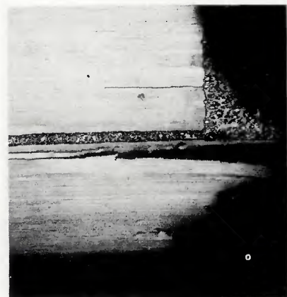
Fig. 13 — Failure of a brazed joint by tearing through the sheet (X50, reduced 54%)
