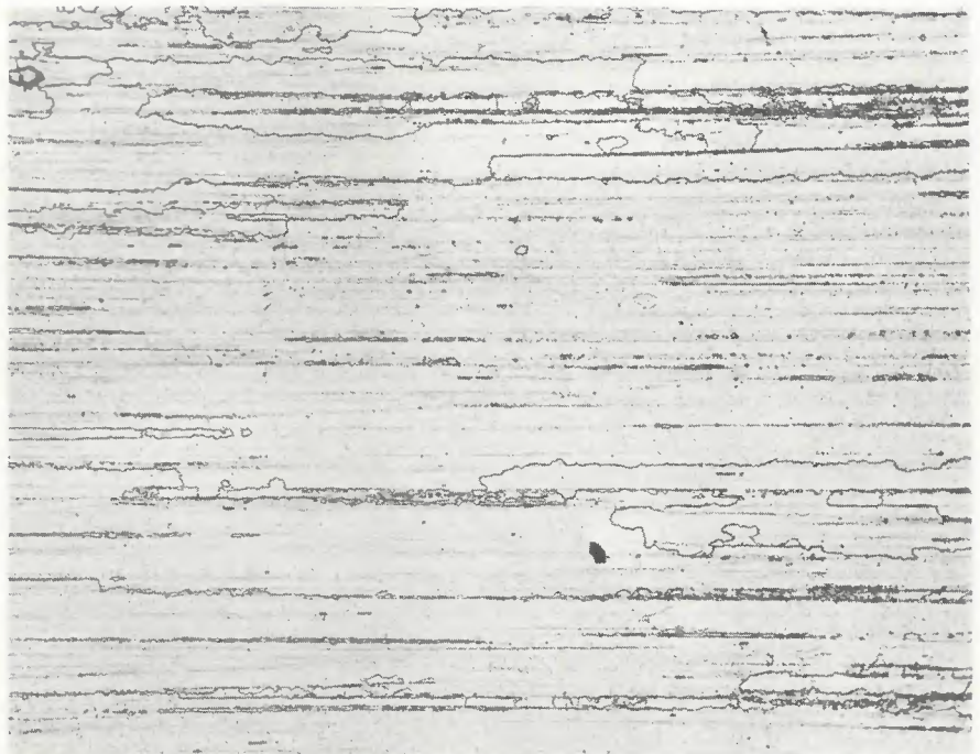
Fig. 4 — Longitudinal cross section of extruded IN-853 (From Ref. 1: X100, reduced 9%)
