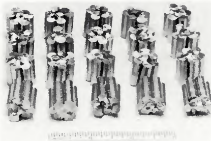
Fig. 1 — Grooved copper mold samples before levitation melting
