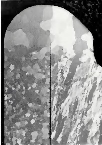
Fig. 4 — Cross section through a weld joining a 1.125 in. OD Tube to a vessel half section. Etchant: 20 vol %  $H_2O_2$ —10 vol %  $H_2SO_4$  (96%  $H_2SO_4$ ) — 70 vol %  $H_2O$ . X29, reduced 49%
