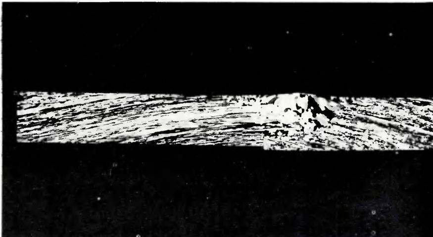
Fig. 6 — Cross section through electron beam girth weld shown in the lead photo. Etchant: 20 vol %  $H_2O_2$  — 10 vol %  $H_2SO_4$  (96%  $H_2SO_4$ ) — 70 vol %  $H_2O$ . X6, reduced 25%
