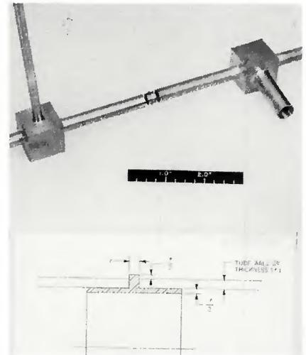
Fig. 9 — (Top) Molybdenum tees with attached tubes and insert in position before assembly for welding. (Bottom) Design of typical insert for 0.250, 0.275, and 0.500 in. OD tube-to-tube welds
