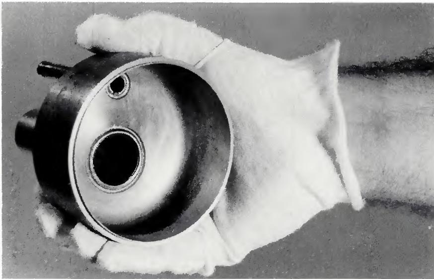
Fig. 2— Back extruded half section with two tube-to-header welds made by the EB process
