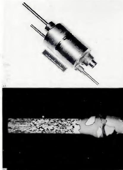
Fig. 5 — (a) Back-extruded molybdenum half sections joined by a manual gas tungsten-arc weld. (b) Cross section through this weld. Etchant: 20 vol %  $H_2O_2$ —10 vol %  $H_2SO_4$  (96%  $H_2SO_4$ ) — 70 vol %  $H_2O$ . X6, reduced 65 %
