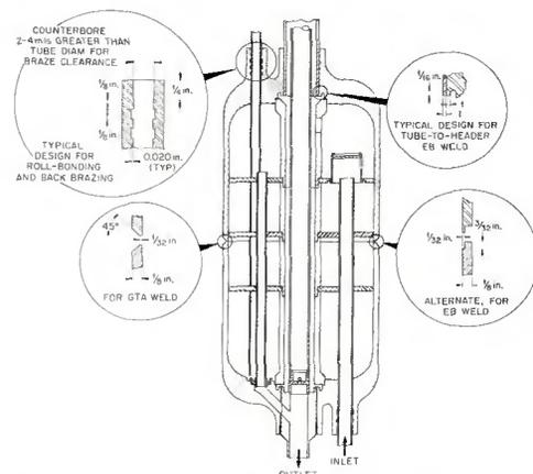
Fig. 1 — Joint designs used in fabricating molybdenum vessels
