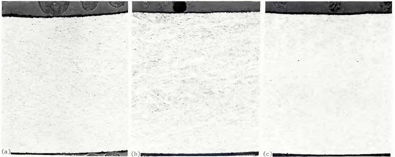
Fig. 11 — Effect of heat treatment (in vacuum) on the microstructure and hardness of 0.500 in. OD  $\times$  0.030 in. wall molybdenum tubing. Etchant: 50 vol %  $\text{H}_2\text{O}_2$ —50 vol %  $\text{NH}_4\text{OH}$ . X100, reduced 24%. (a) As-received, diamond pyramid hardness (DPH)241. (b) 60 min at 900 C, DPH 236. (c) 60 min at 925 C, DPH 206. Note that there is partial recrystallization (resulting in a decrease in hardness) in the sample heat treated at 925 C
