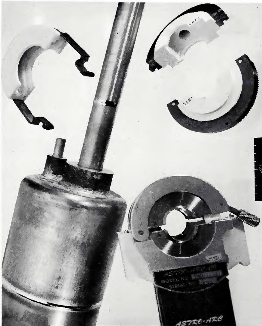
Fig. 7 — Orbiting-arc weld head and 0.875 in. diam tube-to-tube weld
