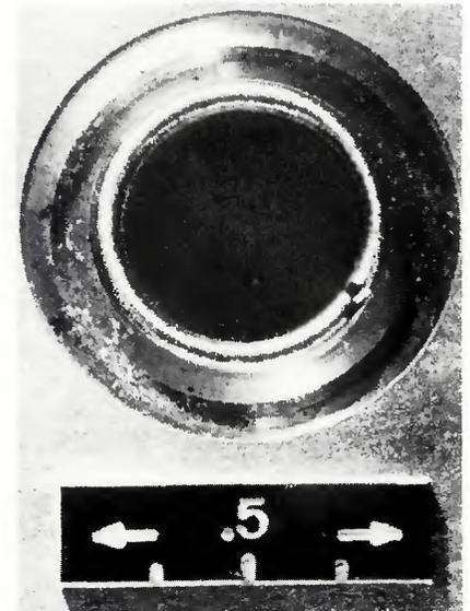
Fig. 3— Closeup of a 0.375 in. diam tube-to-header weld showing the machined groove
