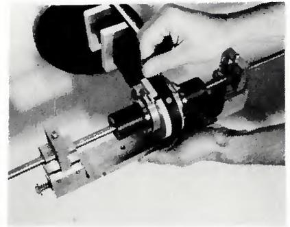
Fig. 8 — Orbiting-arc weld head with attached rubber sleeves for welding molybdenum tubing outside a glove box and with yoke-type fixture
