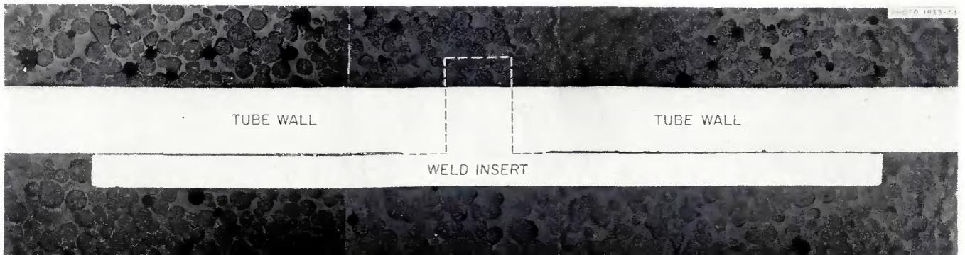
Fig. 10 — Composite of photomicrographs of a cross section through an orbiting-arc field weld joining two 0.250 in. OD  $\times$  0.020 in. wall tubes. Etchant: 50 vol%  $\text{NH}_4\text{OH}$ —50 Vol%  $\text{H}_2\text{O}$  X50, reduced 30%
