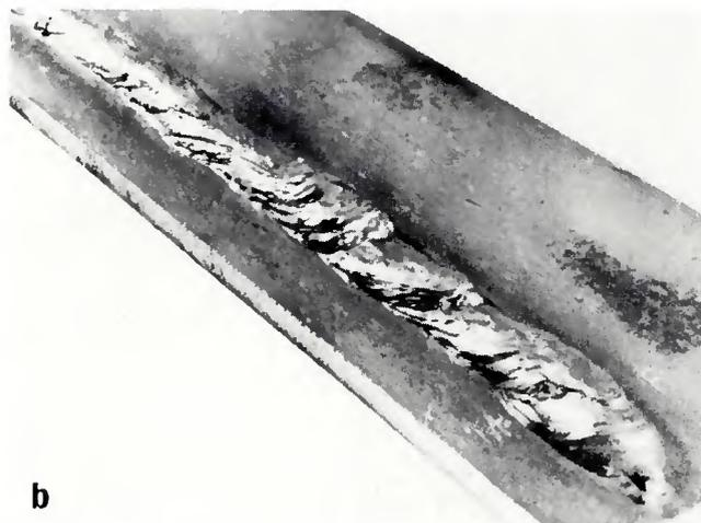
Fig. 9 — (a) Longitudinal penetration characteristics of SAW welds in mild steel with pure  $MgF_2$  flux (electrode positive); (b) surface of SAW weld in mild steel with pure  $MgF_2$  flux (electrode positive)
