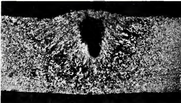
Fig. 1 — GTAW penetration in mild steel with pure MgF<sub>2</sub> flux
