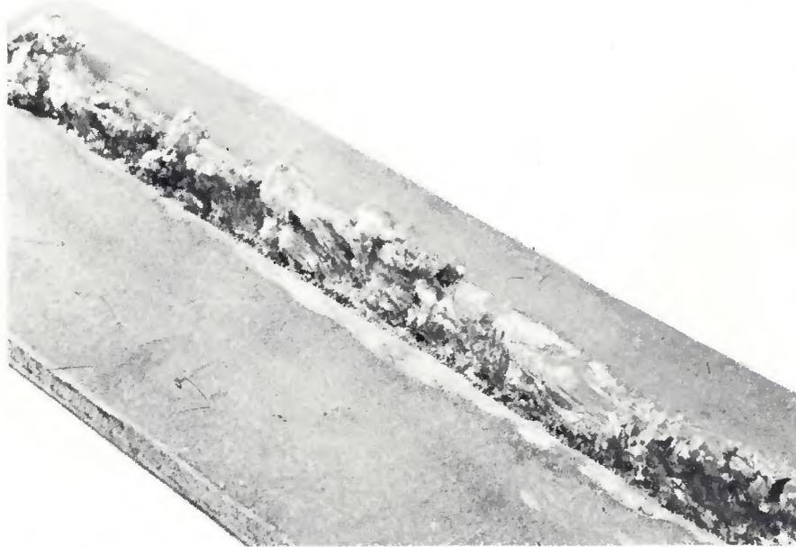
Fig. 7 — Surface of SAW weld in mild steel with pure  $NaF$  flux (electrode negative)
