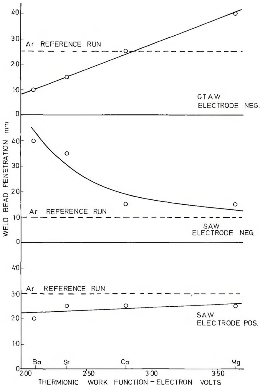
Fig. 11 — Weld penetration in mild steel vs alkaline earth work function for GTAW and SAW welds
