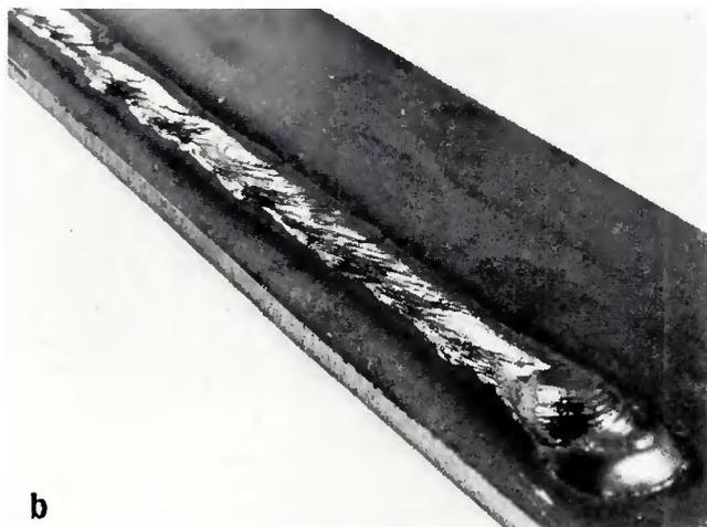
Fig. 10 — (a) Cross-section of SAW weld in mild steel with pure  $BaF_2$  flux (electrode positive); (b) surface of SAW weld in mild steel with pure  $BaF_2$  flux (electrode positive)
