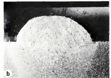
Fig. 8 — Cross-sections of SAW welds in mild steel (electrode negative): (a) 30 mol %  $MgO$  in  $MgF_2$  flux; (b) 30 mol %  $MgO$  in  $BaF_2$  flux
