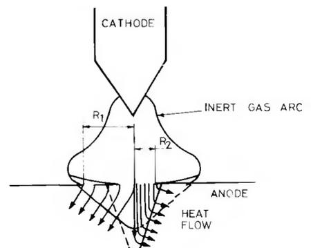
Fig. 12 — Two dimensional model of the relationship between penetration and anode spot size (after Ludwig, Ref. 5)
