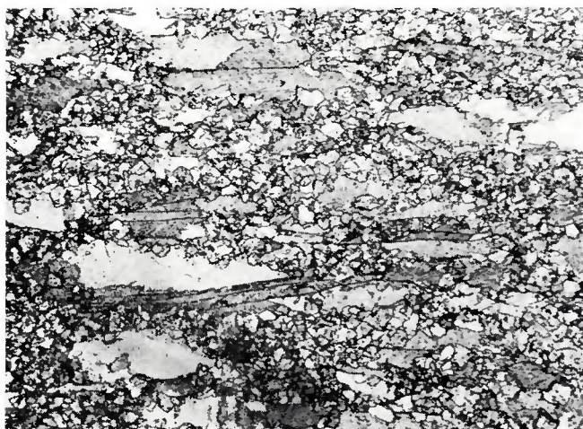
Fig. 1 — Microstructure of grade 300 maraging steel after hot-rolling, solution annealing at 820 C for 4 h, and aging at 480 C for 4 h. An extremely nonuniform structure due to incomplete recrystallization is indicated. (Electrolytic etch with 10% Cr 2 O 3 ; X100, not reduced)
