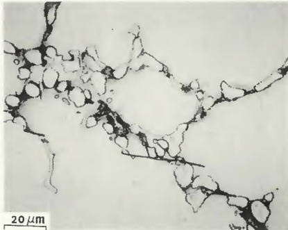
Fig. 1 — Sample heated at 1350 C for 2 h exhibiting large amounts of grain boundary phases
