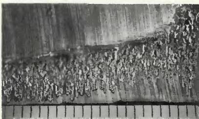
Fig. 6 — Longitudinal section through weld no. 3 (7075 Al). Rule divisions in millimeters
