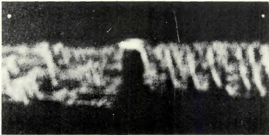
Fig. 8 — Another portion of beam impingement record of weld no. 3 showing one of the infrequent surface closure events. Nominal oscillation frequency, 400 cps. X3.15, reduced 30% (interval between timing dots, 0.050 sec)
