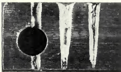
Fig. 9 — Longitudinal section through weld no. 4 (7075 Al). Rule divisions in millimeters
