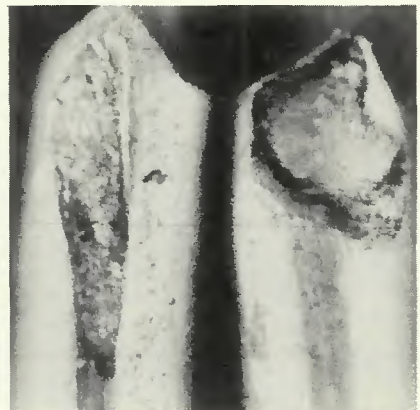
Fig. 15 — Typical faying surface roughness, Sample 2-16-4, X10, reduced 24%. Left, wire-to-wire surface; right die-to-wire surface
