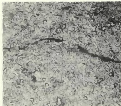
Fig. 5 — Photomicrograph of joint in Sample 7-1-1, plane AA, X400, reduced 32%
