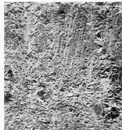
Fig. 7 — Evidence of the solidification structure on the fracture face of a SMA maraging steel weld metal. X60, reduced 31%
