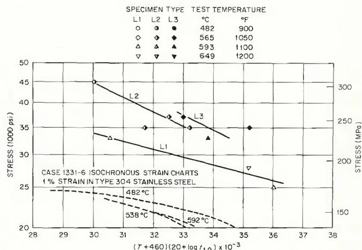
Fig. 4 — Larson-Miller parameter for time to 1.0% strain in CRE type 308 stainless steel weld metal
