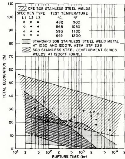
Fig. 6 — Ductility in creep-rupture tests of type 308 stainless steel welds
