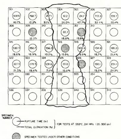
Fig. 8 — Map of rupture times and total elongations for CRE type 308 stainless steel weld metal, Type 304 stainless steel base metal. Hauglass region is weld metal
