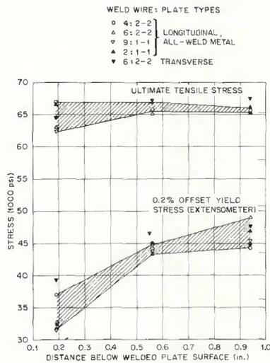
Fig. 2 — Tensile properties of CRE type 308 stainless steel weld metal at 482 C and 0.004/min strain rate. Different batches of welding electrodes and heats of base metal are identified separately (See Table 1)
