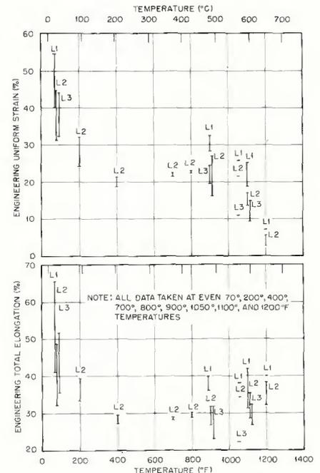
Fig. 3 — Tensile strain properties of type 308 CRE longitudinal all-weld-metal specimens tested at 0.004/min strain rate
