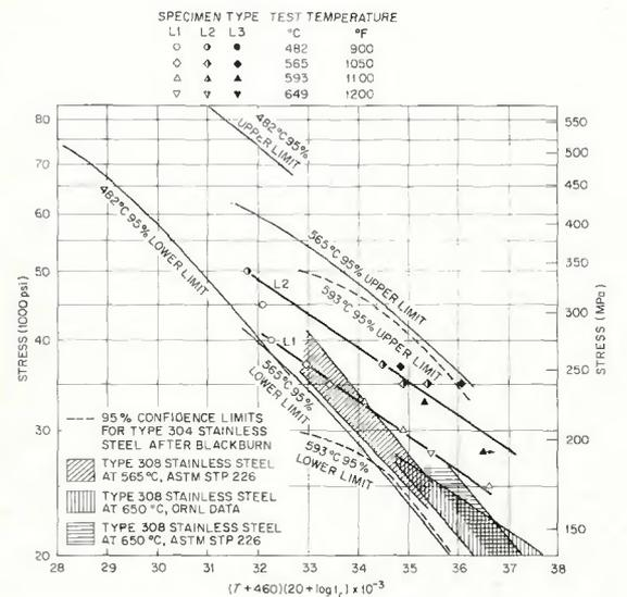
Fig. 5 — Rupture times of CRE type 308 stainless steel weld metal compared with standard weld metal and Type 304 stainless steel base metal, represented by the Larson-Miller parameter
