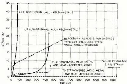
Fig. 7 — Comparison of longitudinal and transverse creep specimens of CRE type 308 stainless steel weld metal at 593 C, 228 MPa (33,000 psi). Failure did not occur in weld metal in transverse specimens
