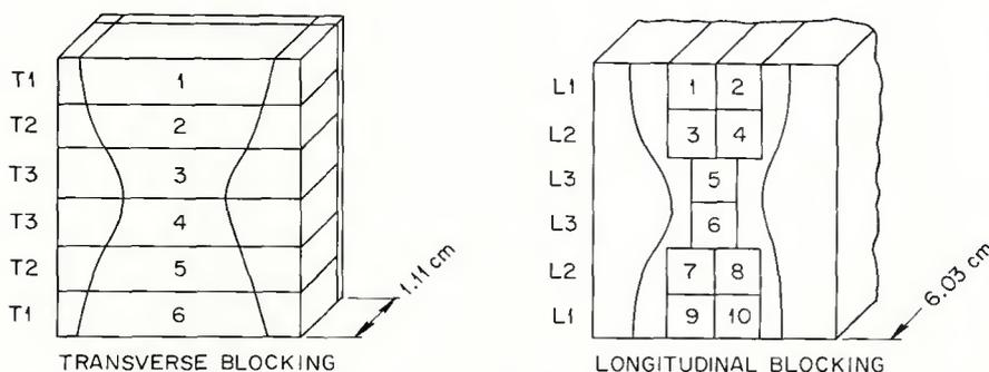
**Fig. 1 — Location and orientation of standard specimens in the test weld. Hour-glass shaped region represents weld metal**
