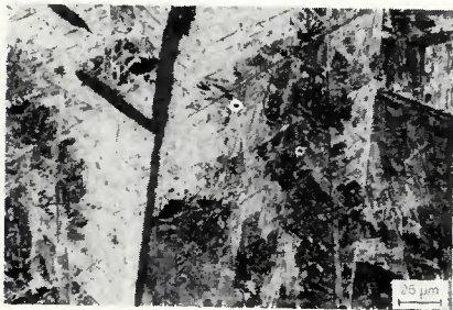
Fig. 10 — Tube B after GTA welding. Longitudinal section of the weld metal. \alpha phase and hexagonal martensite \alpha'' phase
