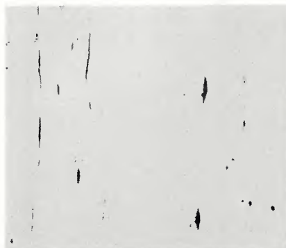
Fig. 8 — Typical array of inclusions used for calibration
