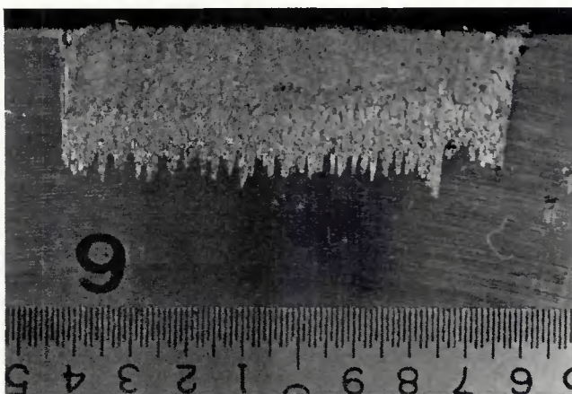
Fig. 11 — Run #9 in Al 7075 made to show spiking obtained without feedback control; 126 kV, 7mA (arbitrary), 21 ipm travel speed (surface focus). X5.94, reduced 46% (scale markings 0.01 in.)
