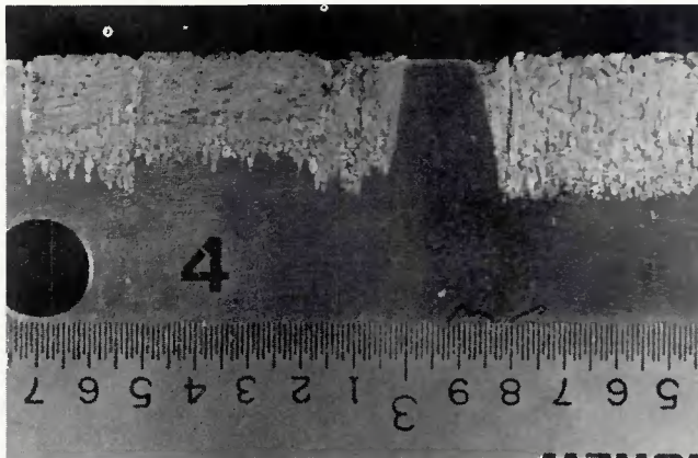
Fig. 9 — Two welds of Run #4 made in Al 7075. Weld at left was made at 5mA (arbitrary). Weld at right was made at 126kV, 7mA, 21 ipm travel speed (surface focus). X4.58, reduced 46% (scale markings 0.01 in.)
