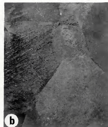
Fig. 5 — Heat-affected zone—(a) direct aged 1100 F-1 h and (b) rolled 20% +1100 F-1 h
