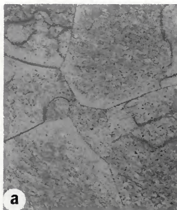
Fig. 5 — Heat-affected zone—(a) direct aged 1100 F-1 h and (b) rolled 20% +1100 F-1 h
