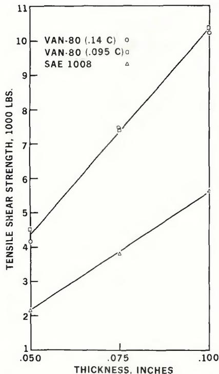
Fig. 9 — Effect of material thickness on the tensile shear strength of spot welds in VAN-80 and SAE 1008 steel
