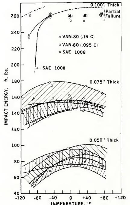
Fig. 16 — Impact shear strength of VAN-80 and SAE 1008 steel spot welds
