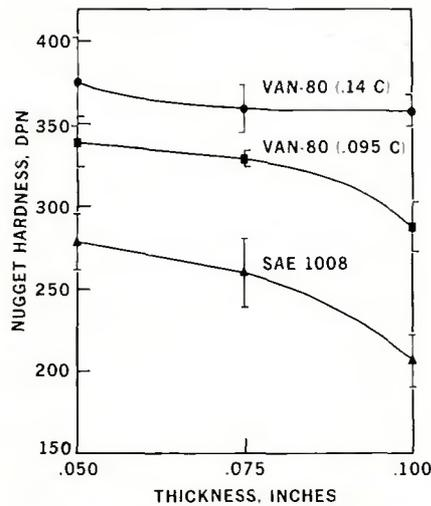
**Fig. 4 — Effect of material thickness on the hardness of VAN-80 and SAE 1008 steel spot welds**
