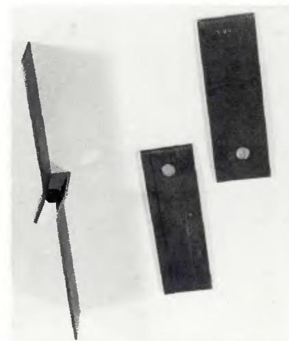
Fig. 10 — Tensile Shear Failures, (left) pull-out failure, and (right) interface failure
