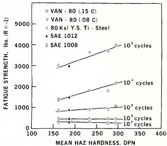
Fig. 21 — Effect of mean HAZ hardness on the fatigue strength of spot welds in 0.073 in. thick material
