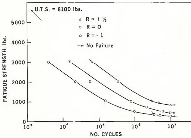
Fig. 17 — Fatigue strength of spot welds in 0.082 in. thick VAN-80(.14C)
