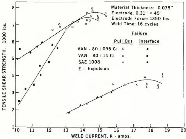
Fig. 6 — Effect of weld current on the tensile shear strength of spot welds in 0.075 in. thick VAN-80 and SAE 1008 steel
