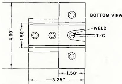
**Fig. 2 — Impact shear specimen and testing jig**
