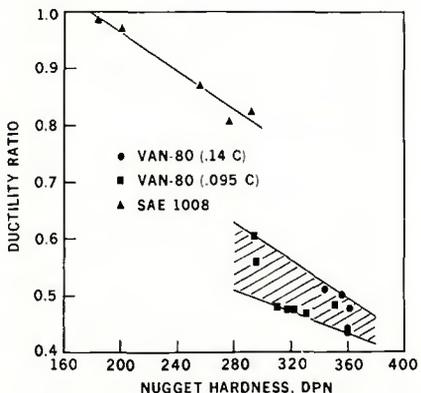
Fig. 15 — Dependence of ductility ratio on weld nugget hardness
