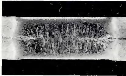
**Fig. 3 — Macrostructure of typical spot weld in VAN-80 Steel. Etchant: 2% Nital; X8, reduced 50%**
