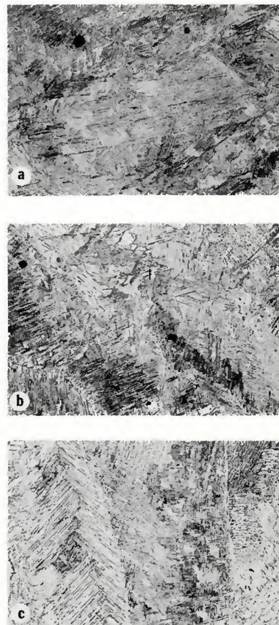
Fig. 5 — Microstructures of weld nuggets in 0.100 in. thick material. (a) VAN-80 (.14C), hardness 360 DPN, predominantly martensitic; (b) VAN-80 (.095C), hardness 293 DPN, mixture of martensite and bainite; and (c) SAE 1008, hardness 207 DPN, mainly bainitic. Etchant: 2% Nital; X500, reduced 52%
