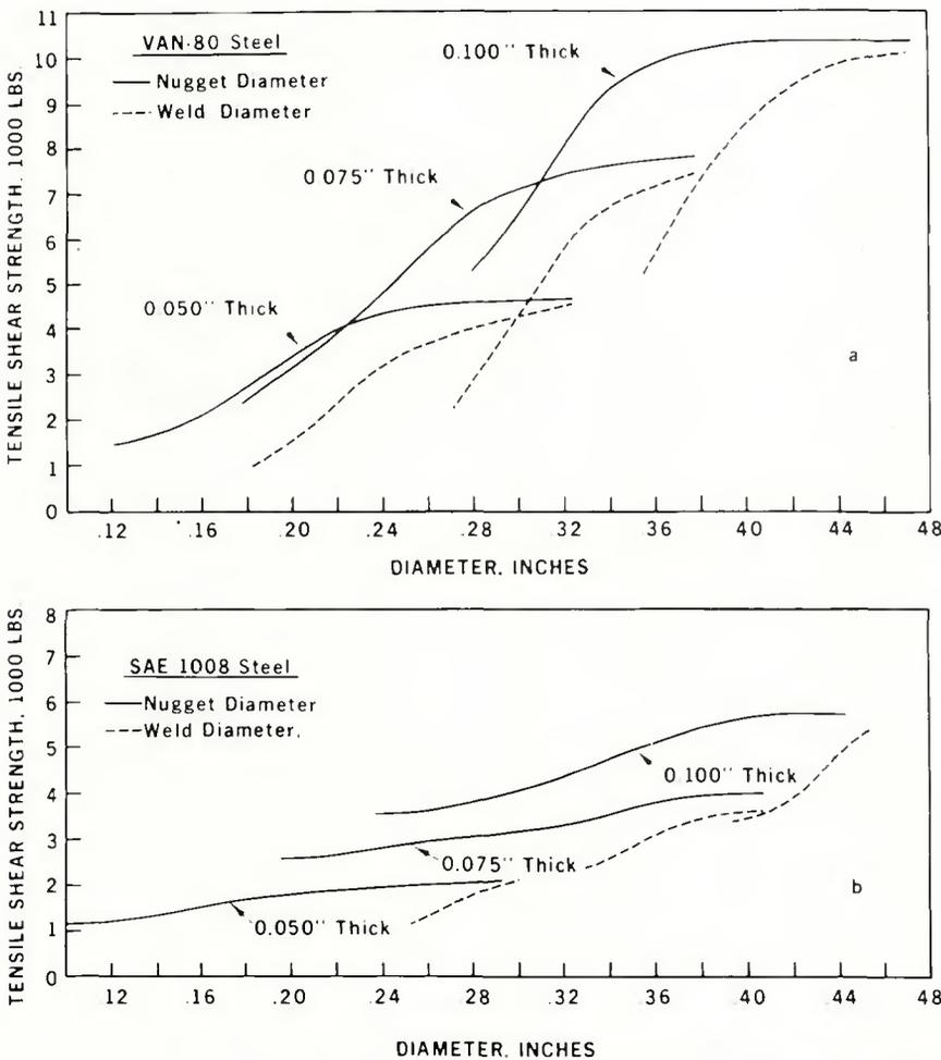
Fig. 8 — Effect of nugget and weld diameters on the tensile shear strength of VAN-80 and SAE 1008 spot welds
