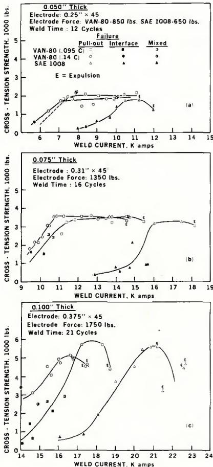
Fig. 13 — Effect of weld current on the cross-tension strength of spot welds in VAN-80 and SAE 1008 steels
