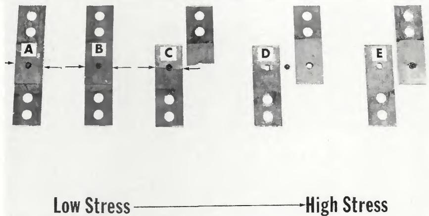
Fig. 19 — Fatigue failures. Arrows indicate failure locations on low stress specimens
