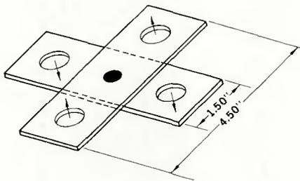
**Fig. 1 — Cross-tension specimen**
