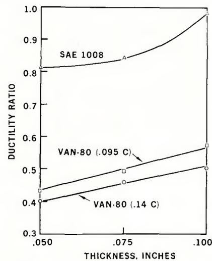
Fig. 14 — Effect of material thickness on the ductility ratio of spot welds in VAN-80 and SAE 1008 steels
