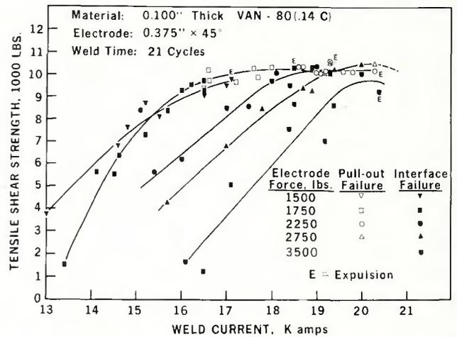
Fig. 7 — Effect of electrode force on the tensile shear strength — weld current relationship for 0.100 in. thick VAN-80 steel
