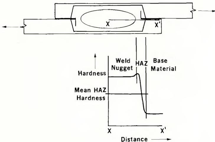
Fig. 20 — Cross-section of spot weld showing hardness profile and location of fatigue cracks
