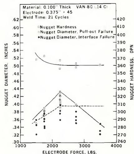
Fig. 12 — Effect of electrode force on the maximum nugget diameter, nugget hardness and the type of failure obtained in the tensile shear test
