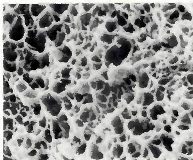
Fig. 11 — Typical fracture surface of a VAN-80 spot weld. X5000, reduced 18%
