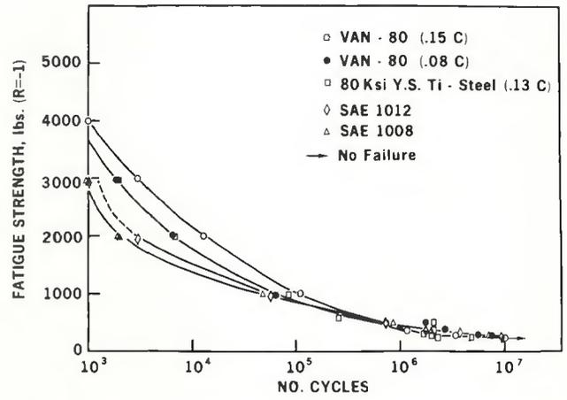
Fig. 18 — Comparison of the fatigue strengths of spot welds in 0.073 in. thick VAN-80 (.08 and .15C), Ti-steel, SAE 1012 and SAE 1008 steels
