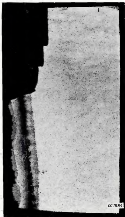
Fig. 3 — Macrosection of fractured bend specimen. The notch tip was located in the base metal but fracture occurred in the weld metal
