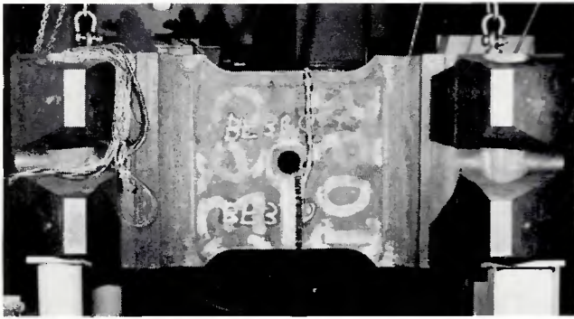
Fig. 12 — Wide plate specimen ready for assembly into the 9,000,000 lb tension test rig
