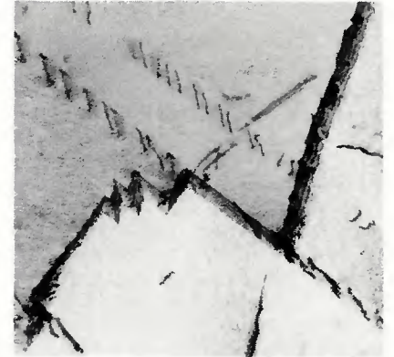
Fig. 10 — Transmission electron micrograph of a solution annealed base metal specimen after an isothermal stress relaxation test at 1400 F X50,000, reduced 29%
