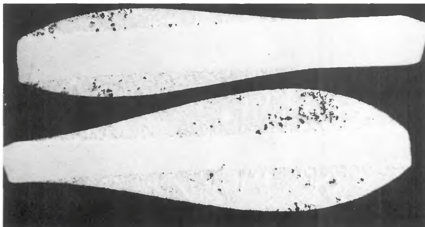
Fig. 6 — Solution of the 3003 alloy core in the drop area, 1/2% HF etch; X9, reduced 52%
