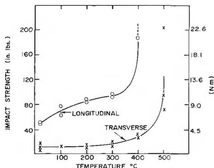
Fig. 3 — Impact test results for TZM
