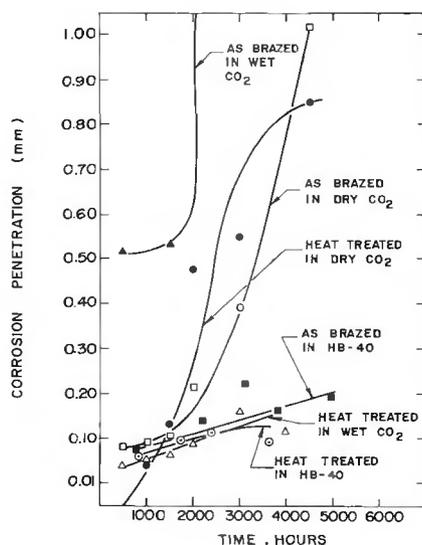
Fig. 6 — Depth of corrosion of braze for TZM/Zr specimen brazed with Zr-5Be
