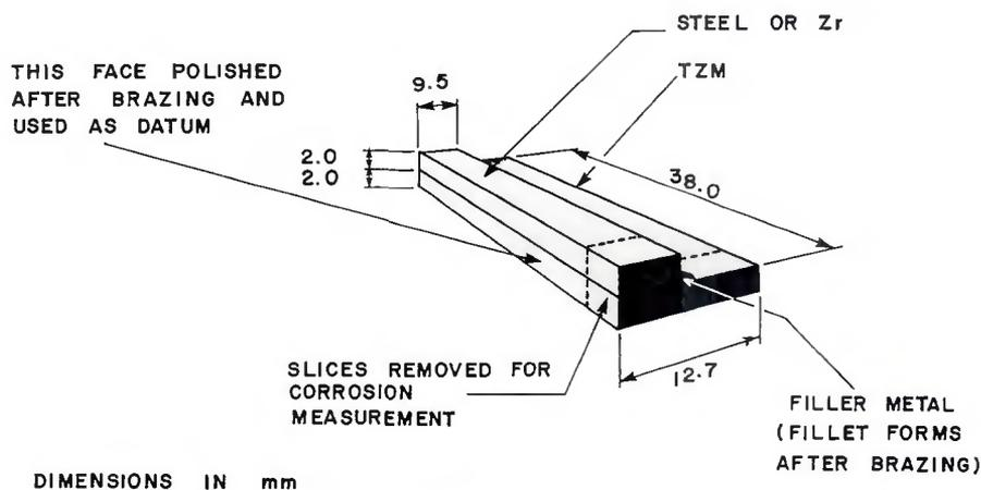
Fig. 5 — Brazed specimen for corrosion testing
