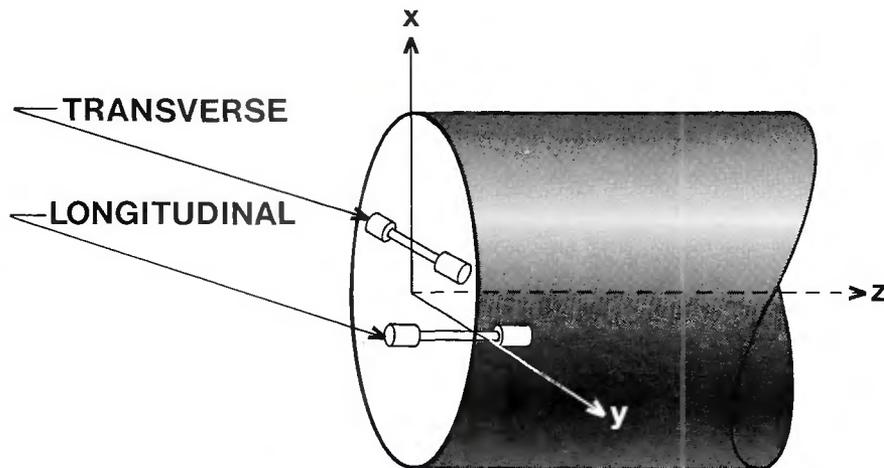
Fig. 2 — Orientation of Instron tensile specimens
