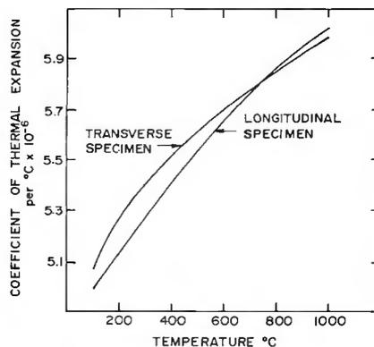
Fig. 4 — Average coefficient of thermal expansion for TZM
