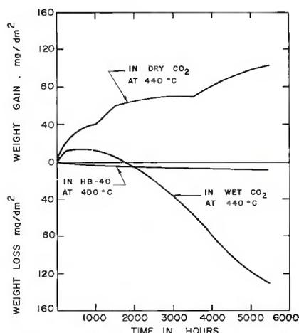
Fig. 1 — Corrosion of TZM
