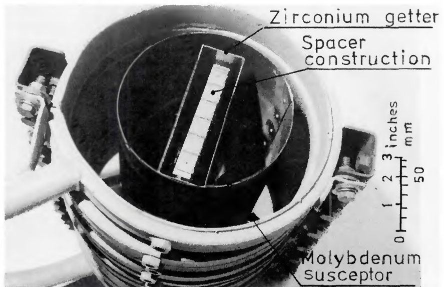
Fig. 6 — Arrangement for getter brazing of the spacer construction shown in the lead photo (title page)
