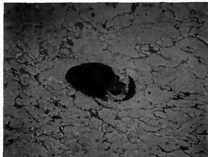
Fig. 1 — An inclusion acting as a microvoid nucleation site in a specimen plastically deformed in uniaxial tension at -51 C. Etchant, 2% nital; X750, reduced 38%
