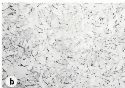
Fig. 7 — Photomicrographs of the refined (a) and unrefined (b) regions of weldment CO. Etchant, 2% nital; X400, reduced 38%
