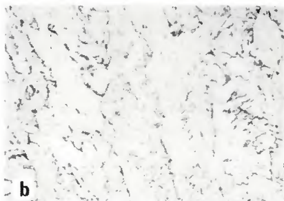
Fig. 6 — Photomicrographs of the refined (a) and unrefined (b) regions of weldment AR. Etchant, 2% nital; X400, reduced 38%
