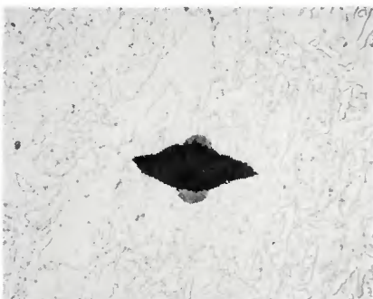
Fig. 3 — An inclusion acting as a crack starter. Specimen deformed in uniaxial tension at -51 C. Etchant, 2% nital; X400, reduced 38%
