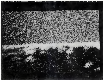
Fig. 1—Example of elemental map for nickel; concentration of nickel in any area is proportional to number of white dots in the area
