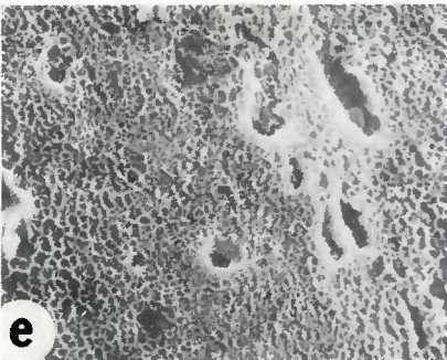
Fig. 7 — Scanning electron photomicrographs showing the change in fracture characteristics for increasing weld input energies of 600, 640, 720 and 760 units (a) to (e) respectively, X2500, not reduced
