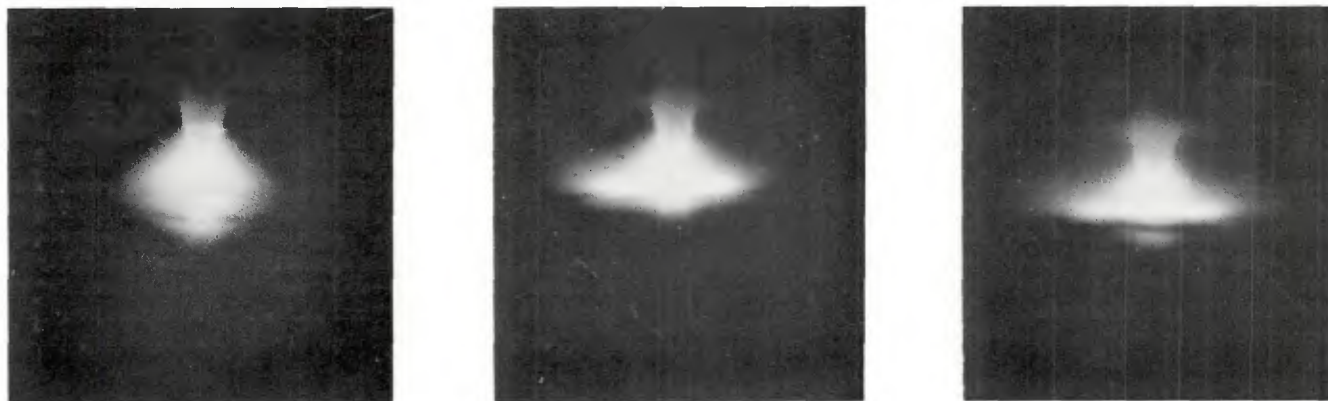
Fig. 9 — Typical arc appearance for a high D/W steel (left), a low D/W steel (center), and a high D/W steel doped with aluminum (right)
