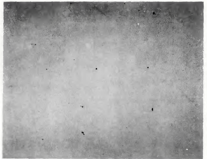
Fig. 5 — Typical inclusion level in an ESR steel. X100, reduced 27%
