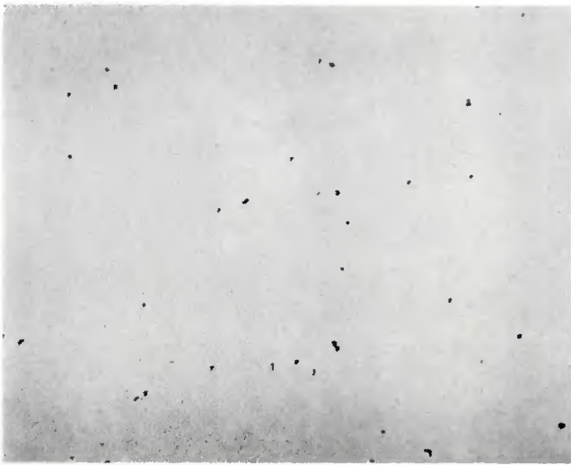
Fig. 4 — Typical inclusion level in an airmelt steel. X100, reduced 27%
