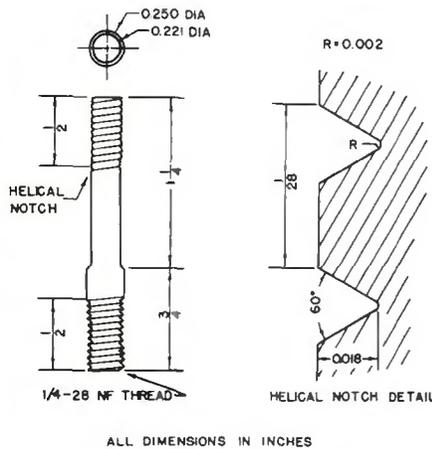
Fig. 3 — Implant specimen details
