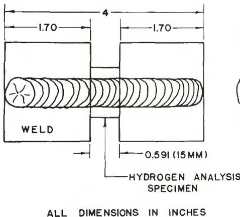
Fig. 4 — Modified hydrogen determination assembly
