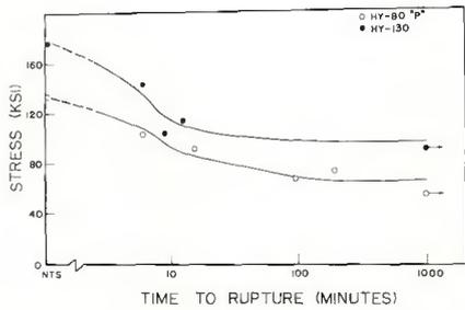
Fig. 9 — Test results of base metal implant specimens loaded in the short transverse direction
