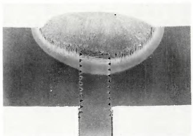
Fig. 5 — Modified implant specimen sectioned near the implant axis. Nital Etch, X3.5, reduced 20%
