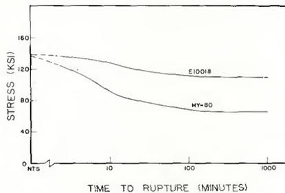
Fig. 12 — Constant-load rupture curves determined from E10018 and HY-80 implant specimens loaded in the short transverse direction
