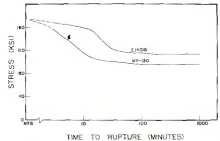
Fig. 13 — Constant-load rupture curves determined from E14018 and HY-130 implant specimens loaded in the short transverse direction
