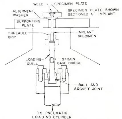
Fig. 6 — Details of implant machine
