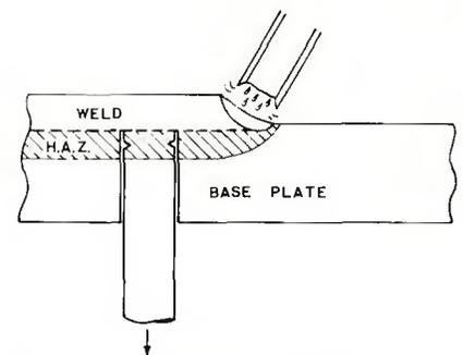
Fig. 1 — Original implant test
