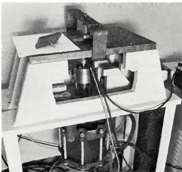
Fig. 7 — Implant machine showing an implant specimen on the left in addition to the specimen loaded under the restraining clamp
