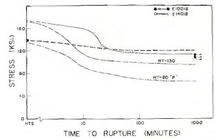
Fig. 11 — Test results of weld metal implant specimens
