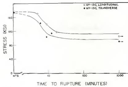
Fig. 10 — Test results of HY-130 implant specimens sectioned in the longitudinal and short transverse directions
