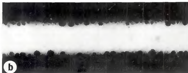
Fig. 7 — Fusion line and general porosity in a copper weld bead deposited at 4 mm/s from a Si-Mn containing filler metal with a 20% N 2 -Ar gas mixture. (a) Macrograph, X5; (b) Radiograph, X1, both reduced 27%
