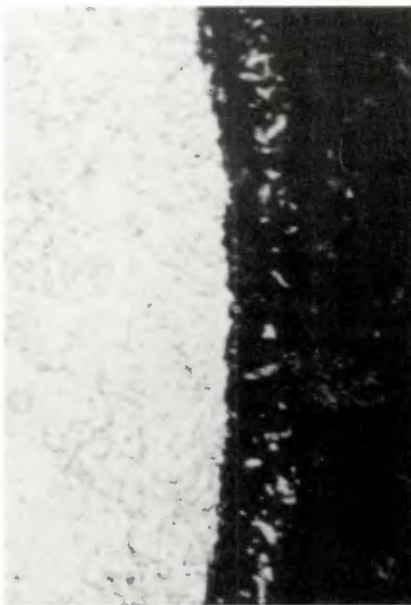
Fig. 10 — Copper-to-solder (80 Pb-20 Sn) interface after 3 min at 900 F showing Cu_3Sn compound particles in solder. X800, reduced 19%
