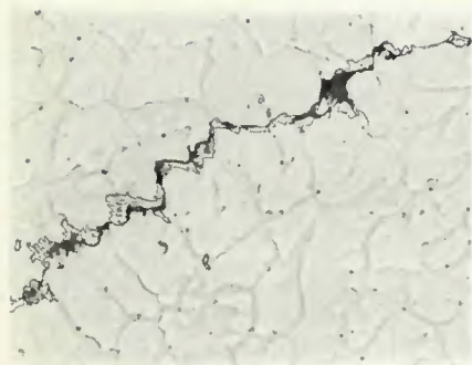
Fig. 7—Liquation cracks obtained in the Vareststraint test with filler metal type 25/22/2.1/N/4.5Mn. \times 800 (reduced 46% on reproduction)
