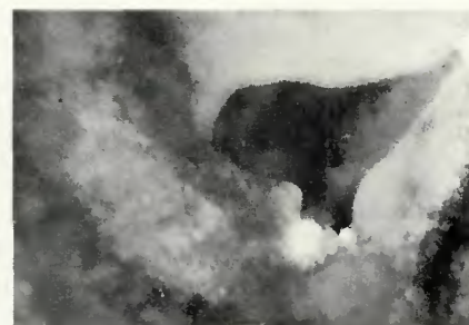
Fig. 4—Sigma phase determined in the structure of the Vareststraint test with filler metal 25/22/2.1/N/4.5Mn. ×21000 (reduced 46% on reproduction)
