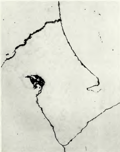
Fig. 7—Microstructure of the joint after one hour aging at 350 C (662 F). \times 400 (reduced 63% on reproduction)
