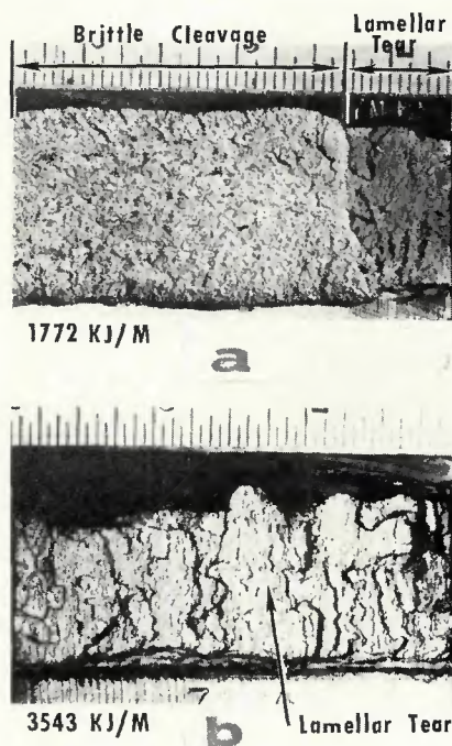
Fig. 3—Fracture appearance at (a) low and (b) high heat input in semi-killed A-285 steel
