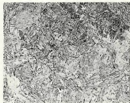
Fig. 7—Microstructure of the synthetic regions, longitudinal section, 1600 F (A—top, \times 750 ) and 2400 F peak (B—bottom, \times 250 ) temperatures. 2% nital etch; reduced 41% upon reproduction
