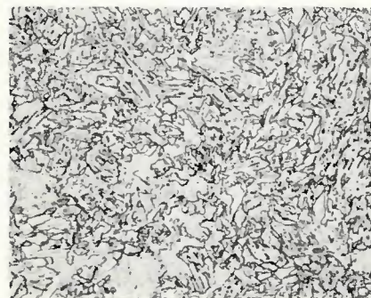
Fig. 10 - Microstructure of the material subjected to 2400 + 1600 F peak temperatures. 2% nital etch; X500 (reduced 41% upon reproduction)
