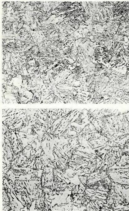
Fig. 9 - Microstructures of the material subjected to double thermal cycles at peak temperatures indicated: A (top) - 2400 and 1150 F; B (bottom) - 2400 and 1350 F. 2% nital etch; X250, reduced 41% upon reproduction
