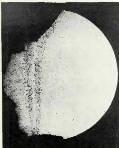
Fig. 10—CVN fracture paths: A (top)—following a plastic hinge 8 kJ/in. (0.31 kJ/mm), -64 C (-83 F), 72 ft-lb (97.6 J); B (bottom)—traveling in weld metal (8 kJ/in. (0.31 kJ/mm), -64 C (-83 F), 18 ft-lb (24.4 J))
