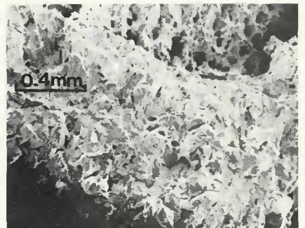
Fig. 12—SEM fractograph of cross weld Charpy test specimen (6 kJ/in. (0.24 kJ/mm), +21 C (+70 F), 48 ft-lb (65.1 J)). The fracture in the weld metal on the lower half of the figure is entirely brittle; the base metal has failed ductilely by void coalescence
