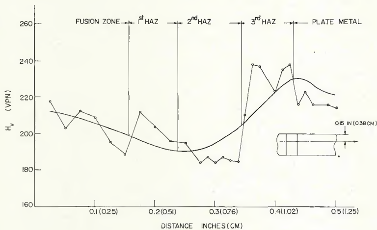
Fig. 4—Microhardness traverse in 35 kJ/in. (1.4 kJ/mm) weld
