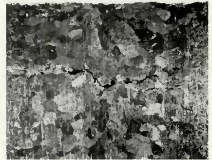
Fig. 6—Crack initiation during longitudinal bend test. \times 7 (reduced 46% during reproduction)
