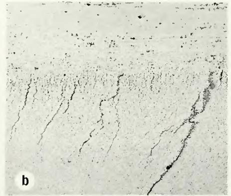
Fig. 9—Completely backfilled fusion zone hot cracks; (a)—lot A specimen, (b)—lot B specimen tested at 4% restraint; Keller's reagent;  $\times 75$  (reduced 36% upon reproduction)
