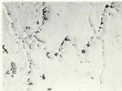
Fig. 12—Liquation of grain boundary regions in the HAZ; electropolish,  $\times 750$  (reduced 50% upon reproduction)
