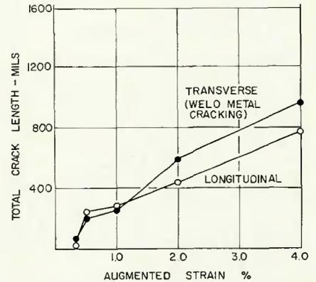
Fig. 4—Total crack length vs. percent augmented strain; lot B welded both transverse and longitudinal to the rolling direction; fusion zone cracking only
