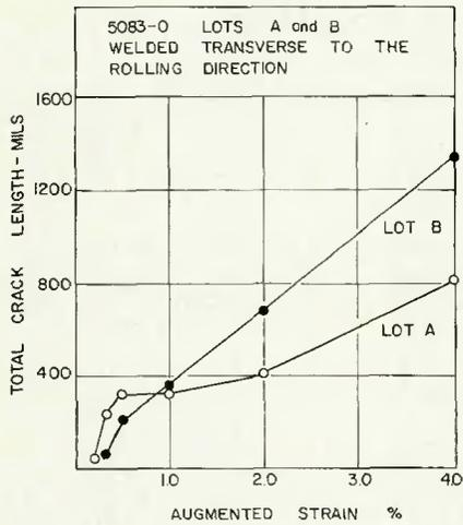
Fig. 2—Total crack length vs. percent augmented strain
