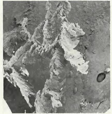
Fig. 14—Epoxy replica of sub-surface fusion zone hot cracks, scanning electron micrograph; X20 (reduced 35% upon reproduction)
