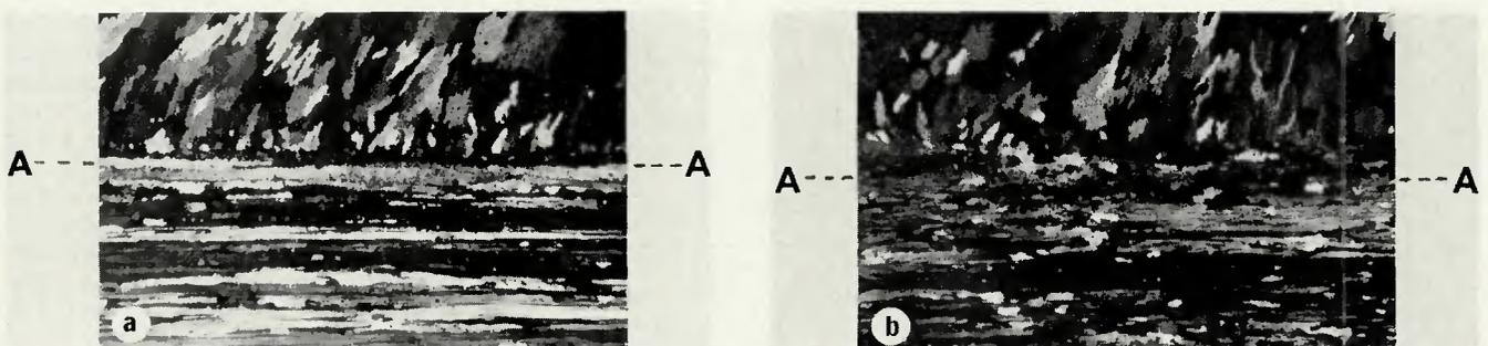
Fig. 5—Grain structure near the fusion line of welded lot B specimens: (a)—welded parallel to the rolling direction; (b)—welded transverse to the rolling direction; electropolish, polarized light,  $\times 70$  (reduced 44% upon reproduction)
