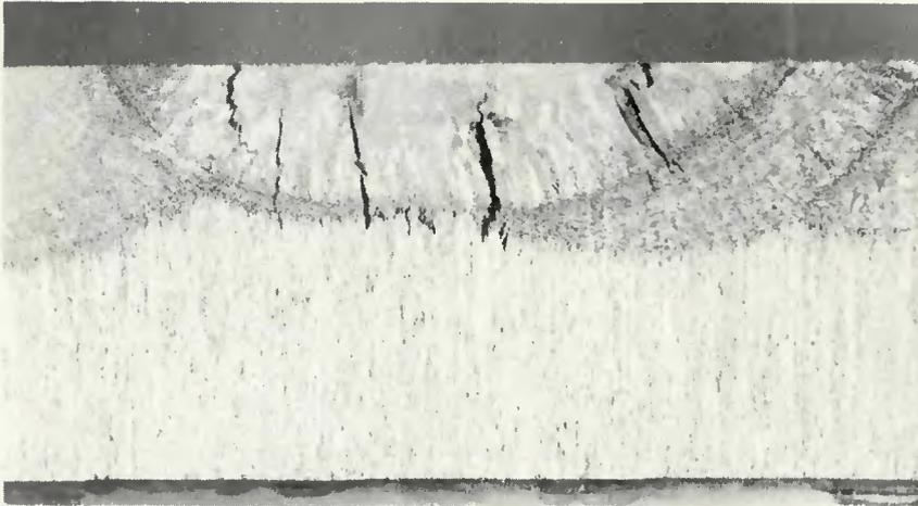
Fig. 13—Subsurface weld hot cracking in a lot A all-weld-metal test specimen, tested at 2% restraint; Tucker's reagent; X4, not reduced
