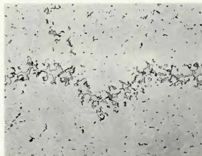
Fig. 10—Backfilled fusion zone hot crack propagating along a grain boundary, lot A specimen; Keller's reagent;  $\times 250$  (reduced 50% upon reproduction)
