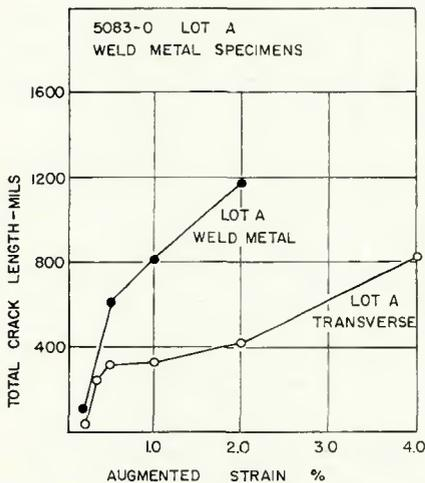
Fig. 6—Total crack length vs. percent augmented strain, lot A specimens welded transverse to the rolling direction compared to all-weld-metal lot A specimens welded under identical conditions
