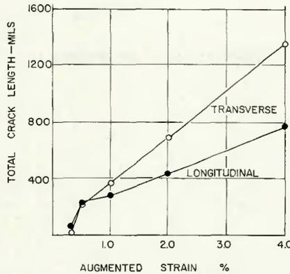
Fig. 3—Total crack length vs. percent augmented strain; lot B welded both transverse and longitudinal to the rolling direction; welded under identical conditions
