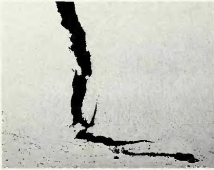
Fig. 8—Typical fusion zone hot crack, lot A specimen tested at 2% restraint; Keller's reagent;  $\times 50$  (reduced 50% upon reproduction)
