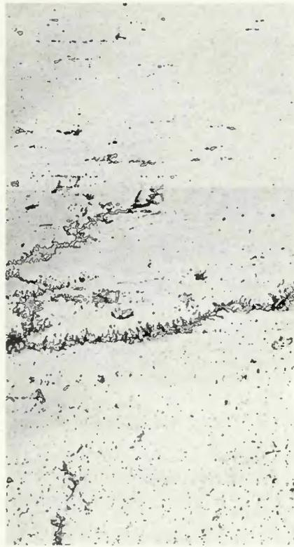
Fig. 11—Panorama illustrating the transition from the base metal to the HAZ to the fusion zone in a lot B specimen, welded transverse to the rolling direction; Keller's reagent;  $\times 150$  (reduced 50% upon reproduction)
