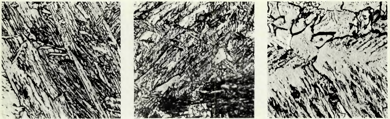
Fig. 12—Comparison of three weld-nugget microstructures: left (a)—Mn-Mo-Cb; center (b)—V-N; and right (c)—SAE 1008 steel. 2% nital, \times 1000
