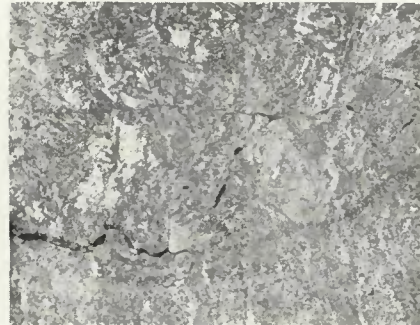
Fig. 5—Cracks in the underwater weld made with E8018 electrode in A537A steel. Nital etch, ×128 (reduced 50% on reproduction)
