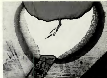
Fig. 14—Underwater weld made with E310-16 electrode in HY-80 Steel. Nital etch, \times 8 (reduced 48% on reproduction)
