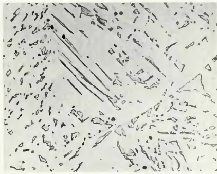
Fig. 7—Micrographs of welds prepared using picral etch: A (top)—weld Bb, showing blocky particles of M-A; B (middle)—weld Bc with blocky M-A particles; C (bottom)—weld Bd with blocky and elongated M-A particles. \times 2000 (reduced 50% on reproduction)
