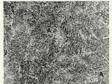
Fig. 6—Micrographs of welds prepared using nital etch: A (top)—weld Bb, cooling rate \Delta t = 190 s, proeutectoid ferrite A and acicular ferrite B; B (middle)—weld Bc, cooling rate \Delta t = 100 s, proeutectoid ferrite A and acicular ferrite B; C (bottom)—weld Bd, cooling rate \Delta t = 30 s, acicular ferrite with regions of coarse bainite A. \times 250 (reduced 50% on reproduction)
