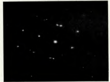
Fig. 8—Identification of M-A particles by T.E.M.: A (top)—weld Bc, with twinned martensite within large M-A particles; B (bottom)—electron diffraction pattern of M-A particles, wherein split spots indicate twinned martensite
