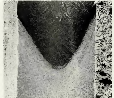
Fig. 6—Shape of the pool revealed in experiment 9 through a sulfur print
