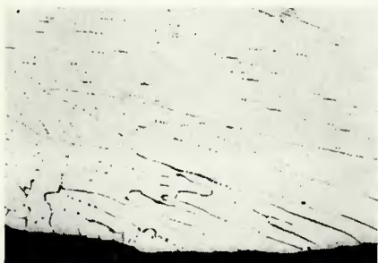
Fig. 7—Oxygen absorption in surface layer of metal at the base of the droplet formed on the end of the filler-metal electrode in GMA weld. \times 400 (reduced 50% on reproduction)
