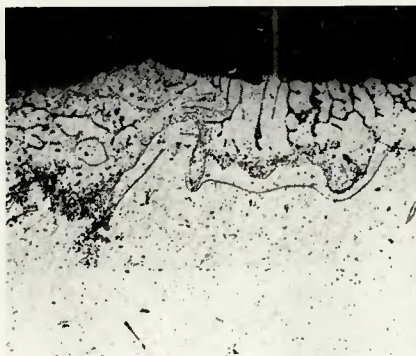
Fig. 13—GMA weld in 2% oxygen-argon atmosphere with 1% aluminum in the filler metal: A (left)—layered surface structure; B (center) region of oxygen absorption at the surface; C (right)—patches of film-like inclusion formations in the body of the weld. \times 120
