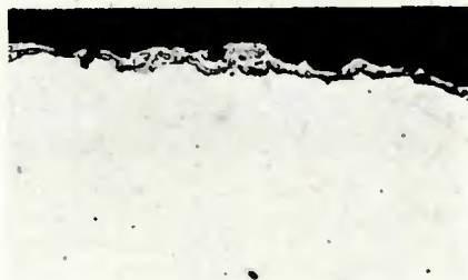
Fig. 10—Reaction layer on droplet surface. \times 600
