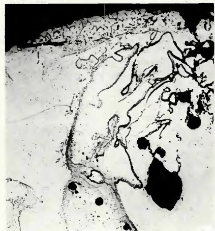
Fig. 11—GTA weld in 2% oxygen-argon atmosphere with 1% aluminum in the filler metal, showing how the reaction becomes more confined to the surface with increasing current: A (left)—100 A, \times 80 ; B (top right)—150 A, \times 120 ; C (bottom right)—200 A, \times 200 (all reduced 30% on reproduction)
