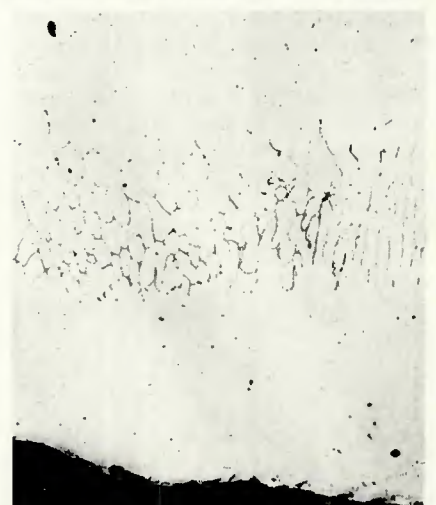
Fig. 3—Oxygen absorption in a GTA weld made in a 2% oxygen-argon atmosphere at 100 amperes. A (top)—high oxygen concentration in surface region, B (bottom)—band of oxygen-rich material, in otherwise low oxygen zone, at base of weld pool. \times 60 (reduced 30% on reproduction)
