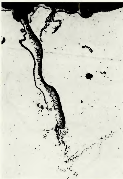
Fig. 12—Aluminum oxide "inclusion streamer" projected into the weld pool from the surface of a GTA weld at 150 A. \times 200 (reduced 30% on reproduction)
