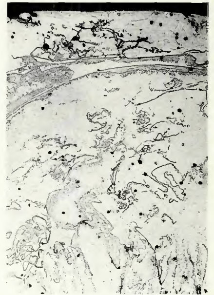
Fig. 16—Weld in tough pitch copper made with filler metal containing 1% aluminum. \times 25 (reduced 30% on reproduction)
