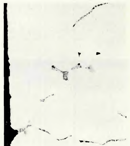
Fig. 17—Inert, insoluble, fluoride flux that has been carried from the surface by the electromagnetically induced motion and trapped in the solidifying ingot. \times 100 (reduced 26% on reproduction)
