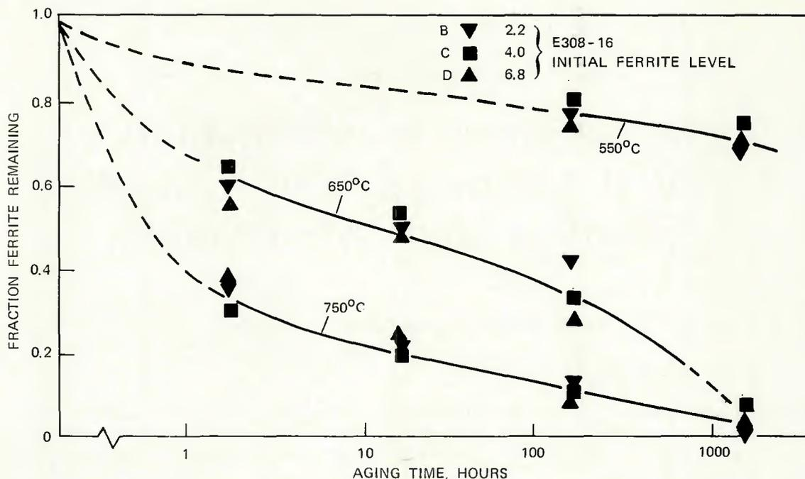
Fig. 2—Fraction of ferrite remaining as a function of aging time for Type 308 stainless steel weld metal
