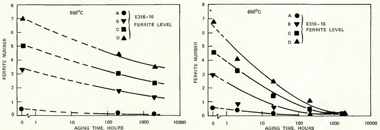
Fig. 1—Ferrite number vs. aging time—Type 316 stainless steel weld metal: A (left)—550 C; B (right)—650 C
